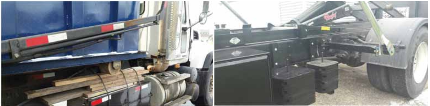
Left: Non-compliant per D.O.T and cumbersome. Right: Clean simple underlayment that is D.O.T compliant.
